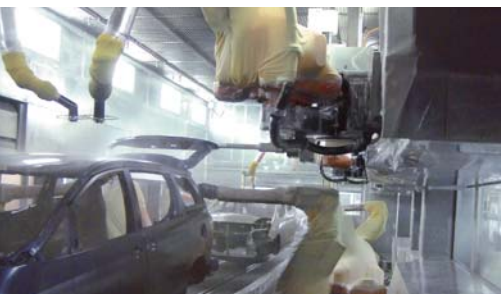
● The new water-borne paint line
