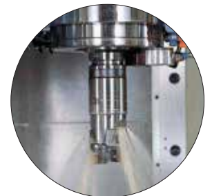
High Pressure Coolant Through Tool
