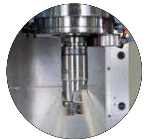
High Pressure Coolant Through Tool
