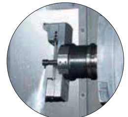
High Pressure Coolant Through Tool
