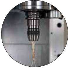
Flange Through (MAX. 1MPa)
