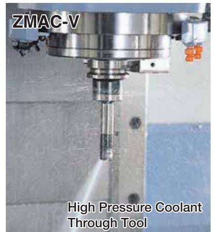
High Pressure Coolant Through Tool
