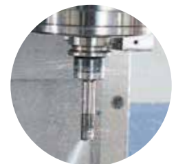
High Pressure Coolant Through Tool
