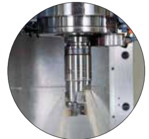
High Pressure Coolant Through Tool
