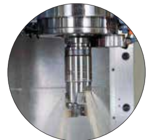
High Pressure Coolant Through Tool
