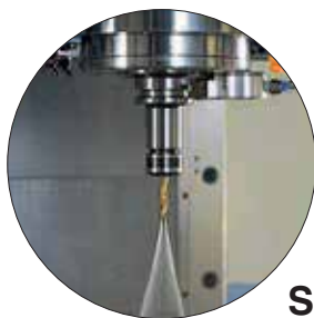
Flange Through (MAX. 1MPa)
