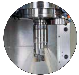
High Pressure Coolant Through Tool
