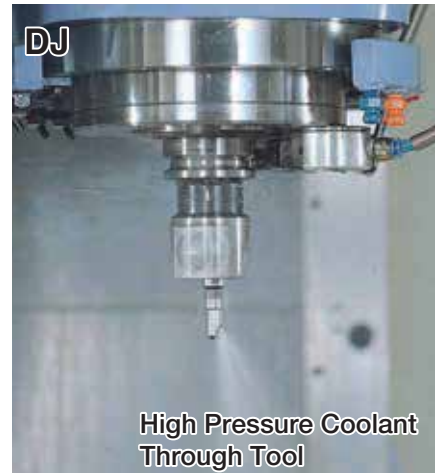
High Pressure Coolant Through Tool
