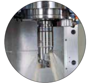
High Pressure Coolant Through Tool
