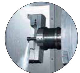
High Pressure Coolant Through Tool
