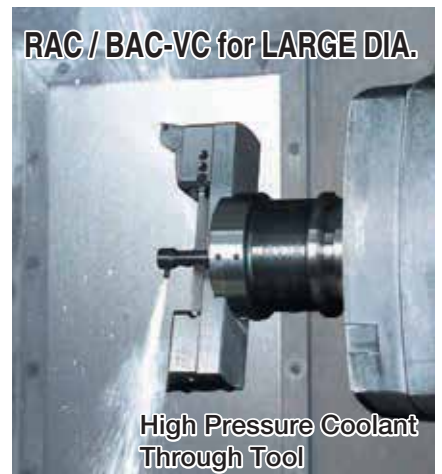
High Pressure Coolant Through Tool
