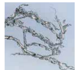
Swarf by reaming blade
