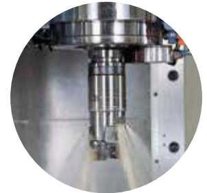
High Pressure Coolant Through Tool
