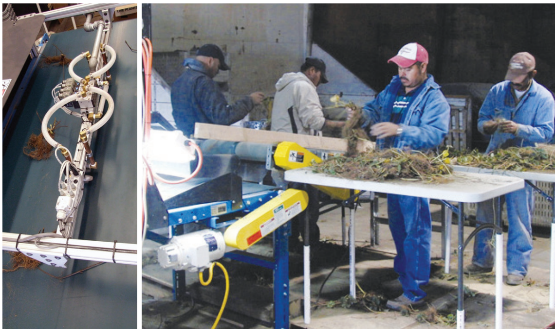
On the field-tested strawberry sorter, air jets (left) blow the classified plants into bins based on quality.
