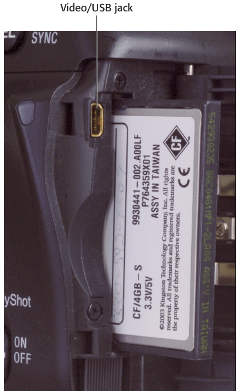
1.13 The video/USB jack enables you to connect your A100 to your video monitor or computer.
