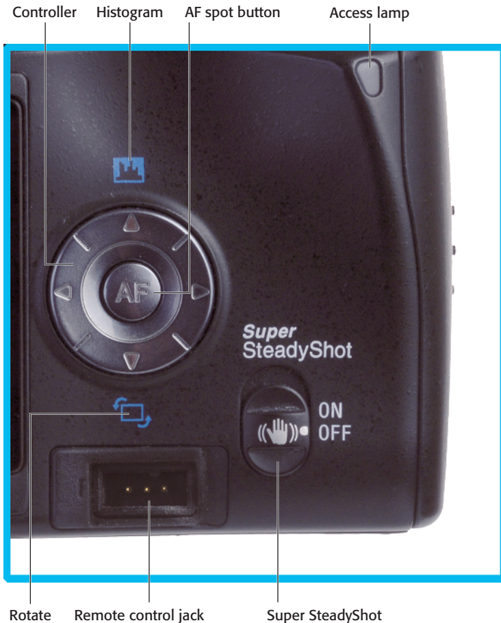
1.12 Key components on the lower-right corner of the back panel of the A100.
