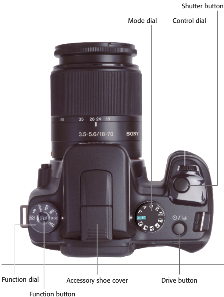
1.7 Key components on the top panel of the A100.
