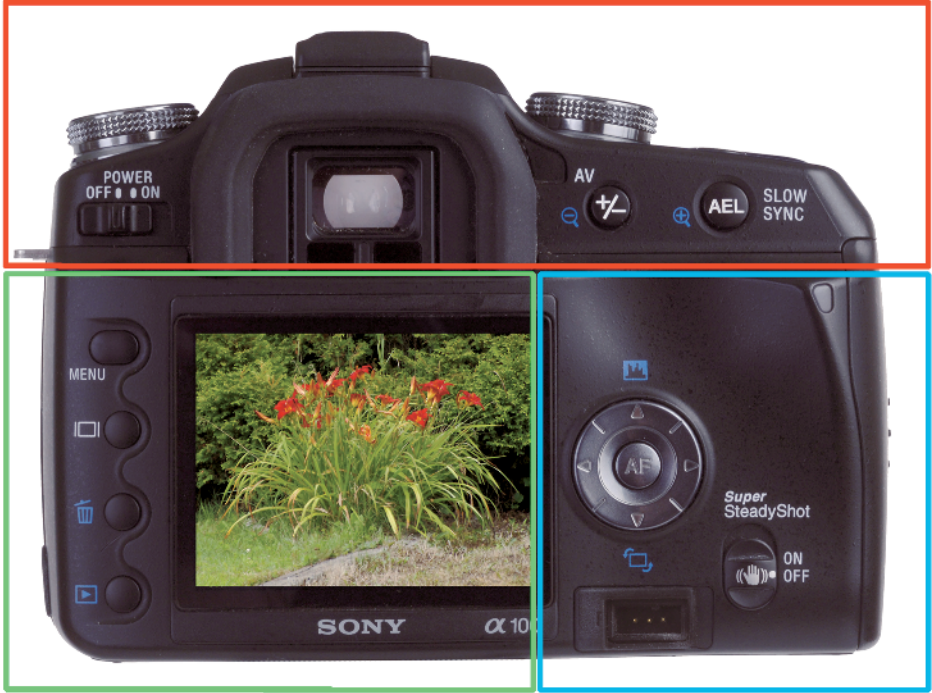
1.8 Key components on the back panel of the A100.
