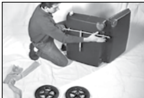
Fig. 3 Attach trailer axle.
