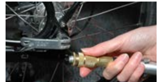
Fig. 12 Trailer hitch connected.
