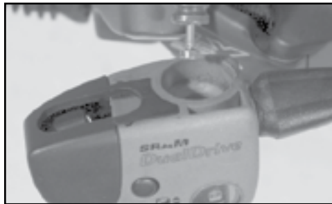
Fig. 7 Place over axle end.
