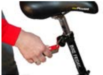
Loosen the seat mast clamp using your 4 mm hex wrench.
